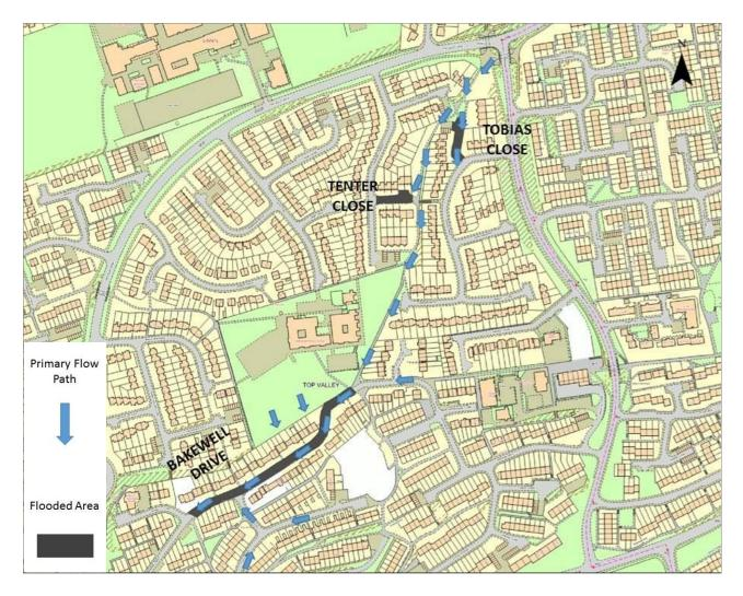
Figure 3: Primary routes of surface water during the flood event. © Crown copyright and database right 2012. Ordnance Survey Licence number 100019317.
