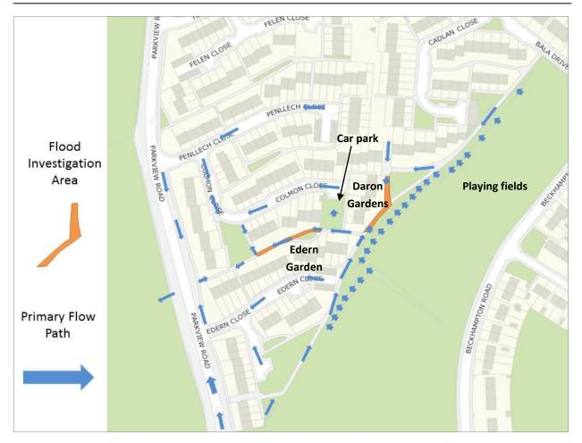
Figure 3: Primary routes of surface water during the flood event. © Crown copyright and database right 2012. Ordnance Survey Licence number 100019317.
