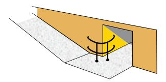
Figure 8.9 Barrier placed at foot of subway ramp
