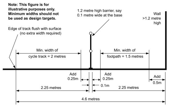
Figure 8.1 Widths for cycle tracks and footpaths
