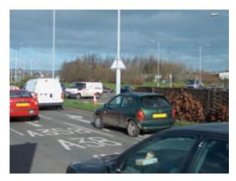
Figure 9.10 Visibility to the right reduced by sight screens (Alex Sully)
