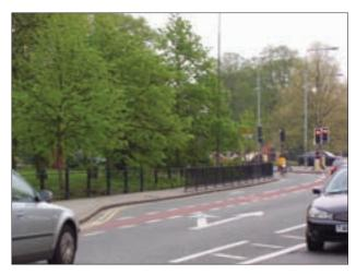
Figure 9.7 Cycle lead-in lane leading to ASL on the off-side of a filter lane (Patrick Lingwood)
