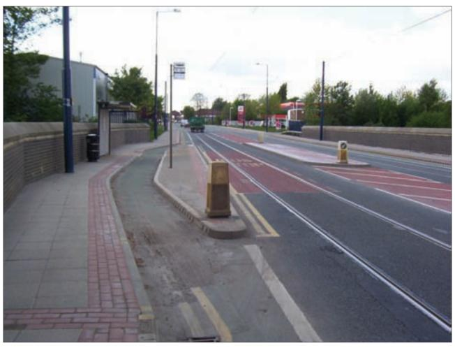
Figure 6.4 Cycle bypass at a bus and tram boarding island. The cycle bypass separates the bus shelter from the boarding area, and this may not be appropriate at busy stops where conflict with boarding and alighting passengers is more likely (Steve Essex)
