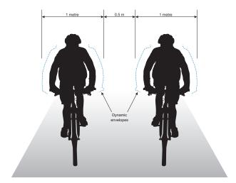
Figure 2.2 Width required by two cyclists
