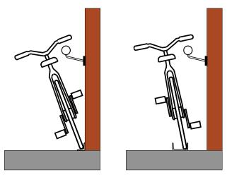
Figure 10.12 Typical wheeling ramp installations
