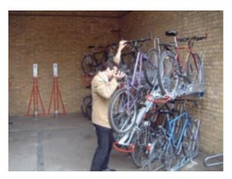
Figure 11.6 Spring-assisted stacking cycle rack (Tony Russell CTC)
