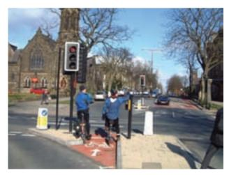
Figure 9.4 Cycle-only phase at signal controlled junction (CTC Benchmarking). Note that the signal head is incorrect, as it uses a red cycle symbol.
