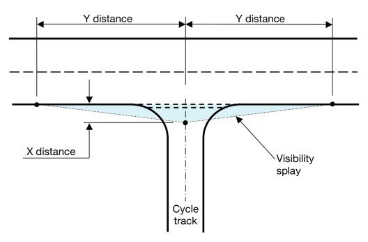
Figure 9.1 Visibility splay measurements
