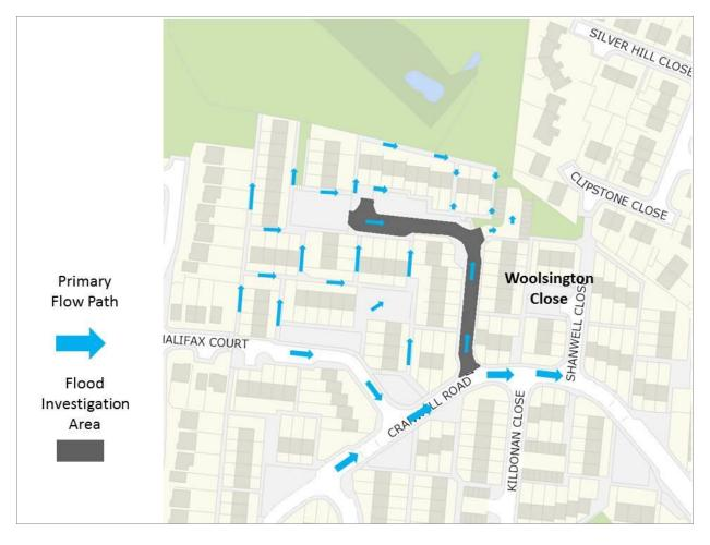
Figure 3: Primary flow routes of surface water during the flood event (based on observed topography). © Crown copyright and database right 2012. Ordnance Survey Licence number 100019317.
